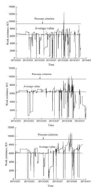
Fig. 1. The support working resistance during first pressure: (a) 25# support of lower work face; (b) 81# support of middle work face; (c) 145# support of middle work face
