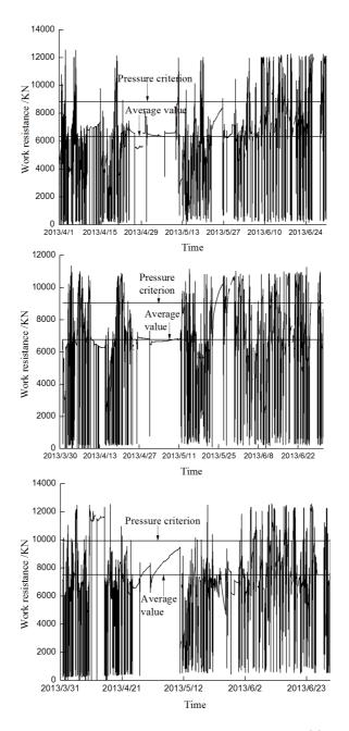
Fig. 2. The support working resistance during periodic pressure: (a) 25# support of lower work face; (b) 81# support of middle work face; (c) 145# support of middle work face
