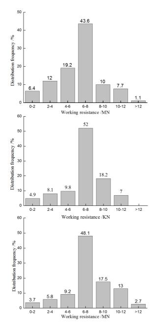
Fig. 3. The distribution frequency of support working resistance: (a) 25# support of lower work face; (b) 81# support of middle work face; (c) 145# support of middle work face
